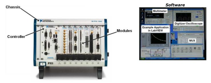
National Instruments PXI-8187 Pentium 4-M 2.5 GHz Embedded Controller. Notice the familiar PC peripherals such as keyboard/mouse and monitor connections, as well as the hard drive, USB 2.0, Ethernet, serial, and other standard PC peripherals. This controller runs standard Windows 2000/XP OSs, or can be targeted with LabVIEW Real-Time.
